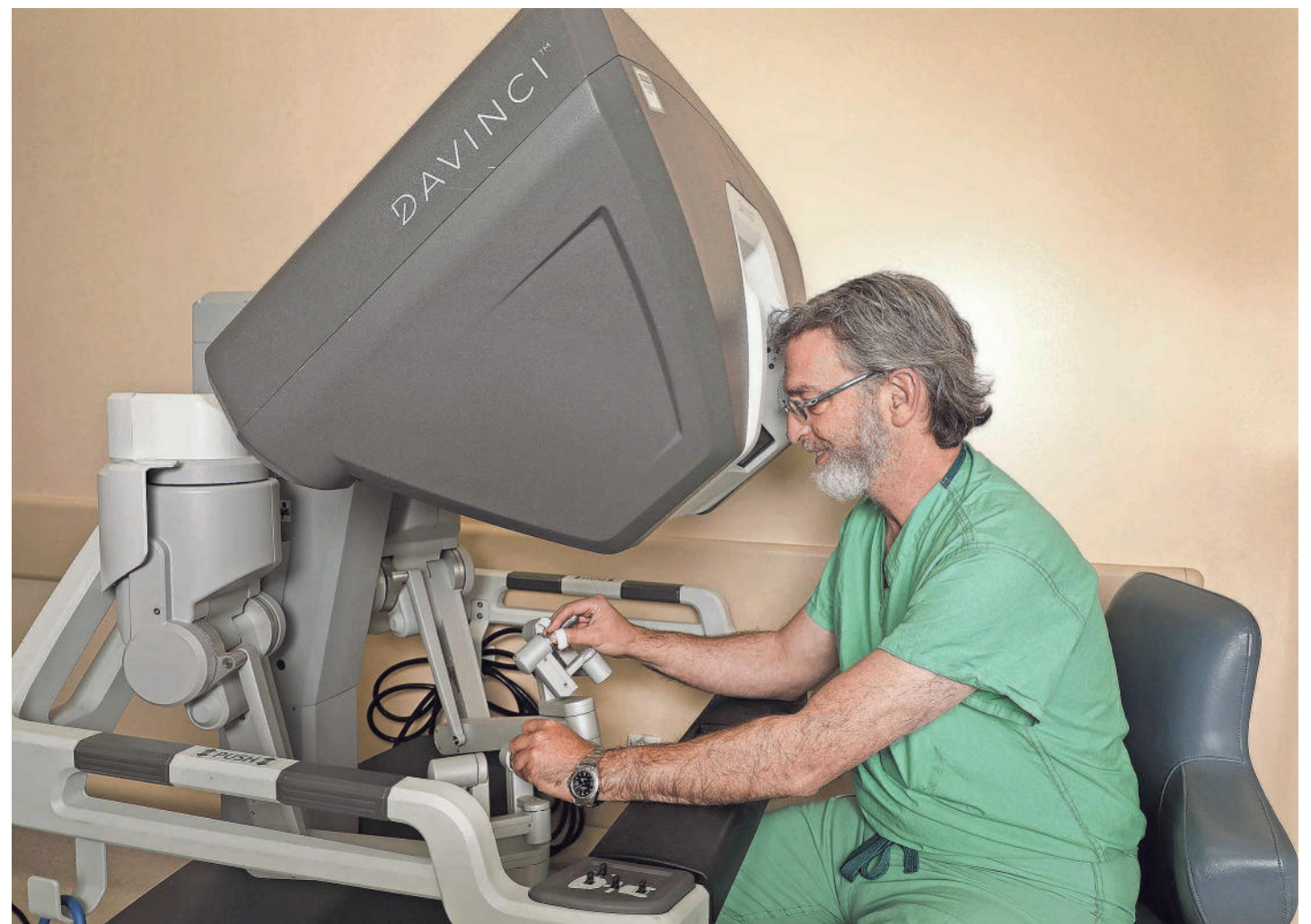
Dr. Ron Landmann, who heads the Baptist MD Anderson Cancer Center's colorectal surgery division in Jacksonville works the controls of the da Vinci robotic surgical system. Dr. Landmann maneuvers the surgical arms with the finger controls while watching the various views of the surgery on the monitor. BOB SELF/FLORIDA TIMES-UNION
